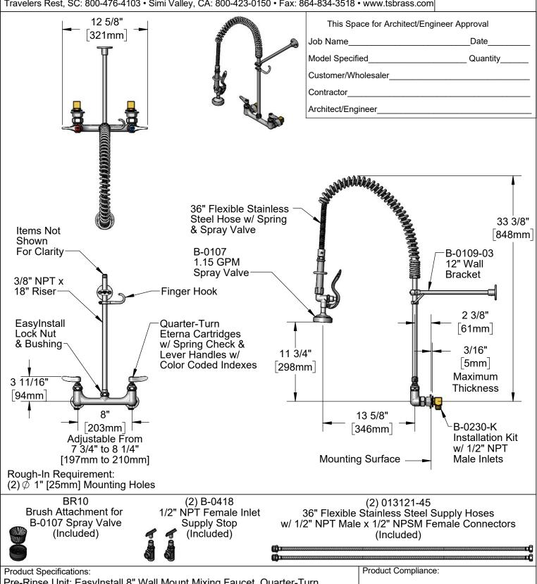
Pre-Rinse Unit: EasyInstall 8" Wall Mount Mixing Faucet, Quarter-Turn Eterna Cartridges w/ Spring Checks, Lever Handles, 36" Flexible Stainless Steel Hose, 1.15 GPM Spray Valve w/ Brush Attachment, Installation Kits w/ 1/2" NPT Male Inlets, (2) 36" Flexible Stainless Steel Hoses & (2) 1/2" NPT Female Supply Stops
