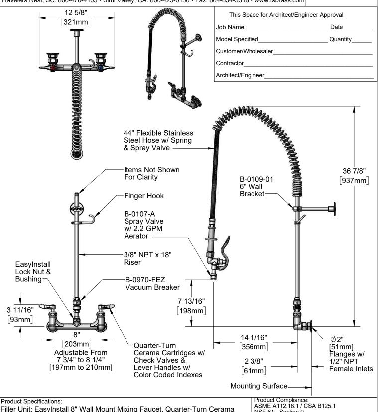
Filler Unit: EasyInstall 8" Wall Mount Mixing Faucet, Quarter-Turn Cerama Cartridges w/ Check Valves, Lever Handles, 44" Flexible Stainless Steel Hose, Spray Valve w/ 2.2 GPM Aerator, Vacuum Breaker, 6" Wall Bracket & 1/2" NPT Female Inlets
