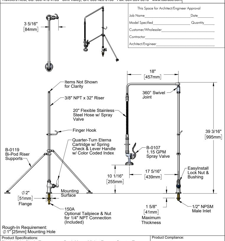
Single Hole, Single Temperature Deck Mount Mixing Faucet, Quarter-Turn Eterna Cartridge w/ Spring Check, Lever Handle, 18" Overhead Swivel Arm, Bi-Pod Riser Supports, 20" Flexible Stainless Steel Hose, 1.15 GPM Spray Valve & 1/2" NPSM Male Inlet
