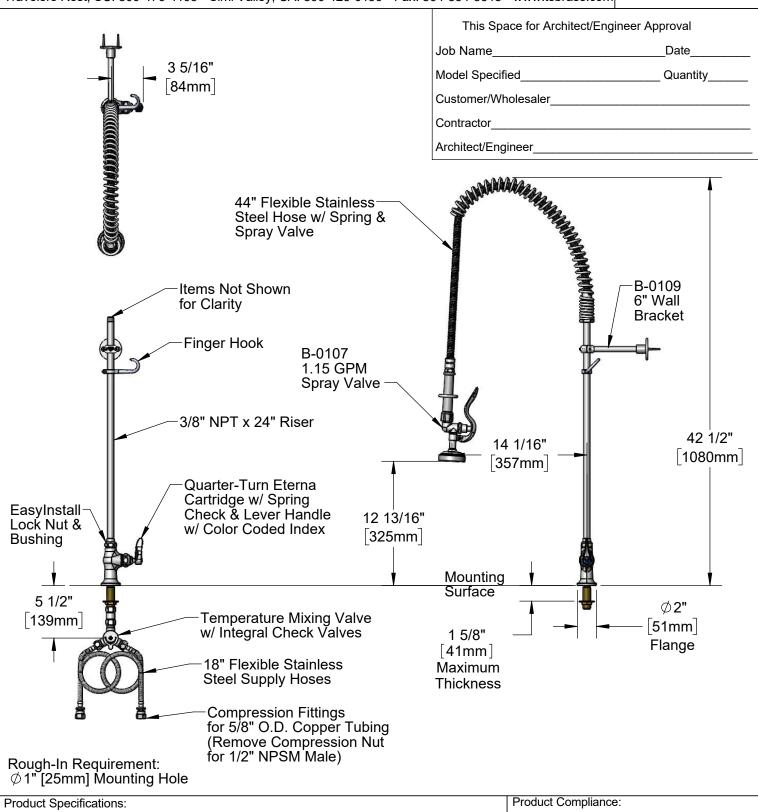
Pre-Rinse Unit: Single Hole, Single Temperature Deck Mount Faucet, Quarter-Turn Eterna Cartridge w/ Spring Check, Lever Handle, 24" Riser, Wall Bracket, 44" Flexible Stainless Steel Hose, 1.15 GPM Spray Valve, Temperature Control Mixing Valve w/ Integral Check Valves & 18" Flexible Stainless Steel Supply Hoses w/ 1/2" NPSM Male Inlets
