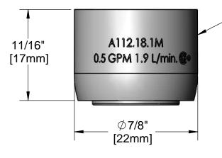
B-0199-01-N05 0.5 GPM [1.9 L/min] Non-Aerated Spray Device, 55/64"-27 UN Female Thread
