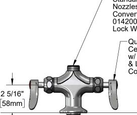
Swivel Outlet Accepts Standard T&S Swing Nozzles. Converts to Rigid w/ 014200-45 Lock Washer (Included).
