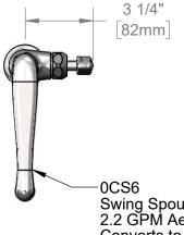
Swing Spout w/ 2.2 GPM Aerator. Converts to Rigid w/ 014200-45 Lock Washer (Included)
