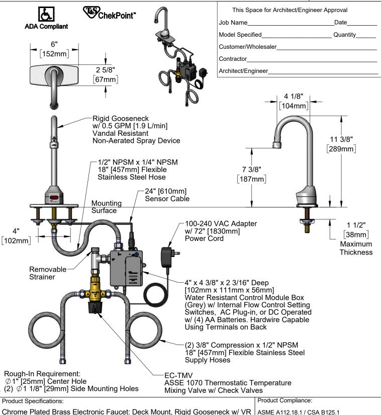
Chrome Plated Brass Electronic Faucet: Deck Mount, Rigid Gooseneck w/ VR 0.5 GPM Non-Aerated Spray Device, 4" c/c Deck Plate, AC/DC Control Module w/ Internal Flow Control Setting Switches, Thermostatic Temperature Control Mixing Valve w/ Check Valves, 18" Supply Stop Flexible Connector Hoses
