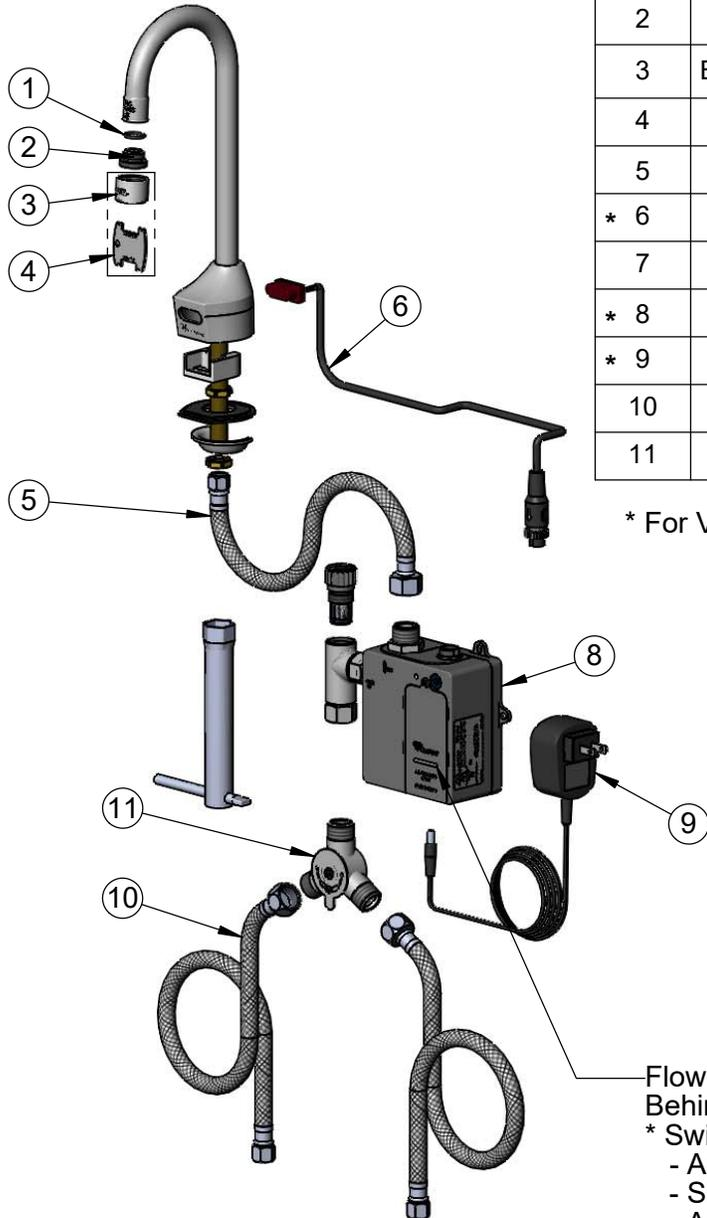
A Maximum of (8) ChekPoint Faucets can be Hardwire Connected and Powered by EC-HARDWIRE ChekPoint Hardwire AC Transformer. (Sold Separately)
