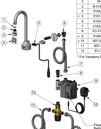
ITEM SALES NO. **DESCRIPTION** NO. 1 006575-45 O-Ring 2 044A 3/8" to Aerator Adapter B-0199-06 Aerator, Vandal Resistant 015425-45 Vandal Resistant Key 019174-45 Sensor Cable Assembly 015345-20 Short Elbow, 3/8 NPSM Flex Connector, 3/8 NPSM x 1/2 NPSM 016325-45 **EC-FILTER** Replacement Filter 019944-45 ChekPoint Control Module w/ Filter Tee 5EF-0002C AC Adapter - US Plug 5EF-0005 Supply Hose, 9/16-24 Female x 1/2" NPSM EC-TMV ASSE 1070 Thermostatic Mixing Valve
