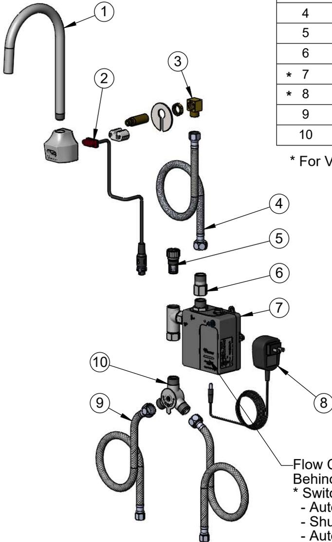
Flow Control Switches are Located Behind Battery Compartment Cover.
