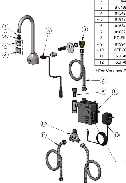
ITEM SALES NO. **DESCRIPTION** NO. 1 006575-45 O-Ring 2 044A 3/8" to Aerator Adapter B-0199-06 Aerator, Vandal Resistant 015425-45 Vandal Resistant Key 019174-45 Sensor Cable Assembly 015345-20 Short Elbow, 3/8 NPSM Flex Connector, 3/8 NPSM x 1/2 NPSM 016325-45 **EC-FILTER** Replacement Filter 019944-45 ChekPoint Control Module w/ Filter Tee 5EF-0002C AC Adapter - US Plug 5EF-0005 Supply Hose, 9/16-24 Female x 1/2" NPSM 5EF-0006 Temperature Mixing Valve
