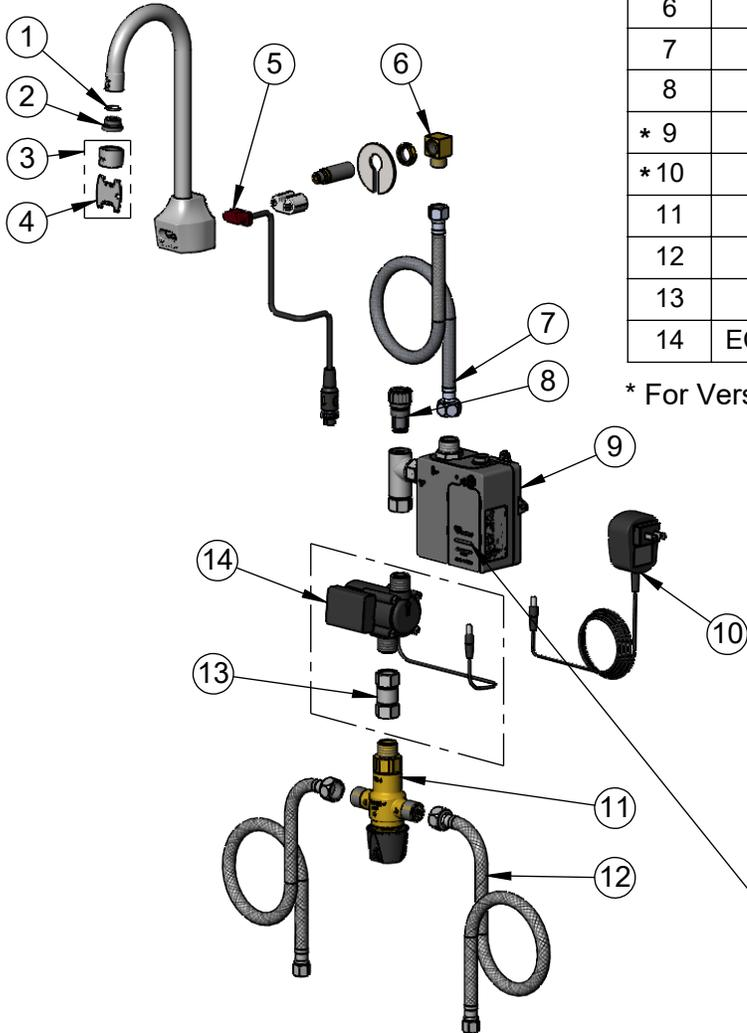
A Maximum of (8) ChekPoint Faucets can be Hardwire Connected and Powered by EC-HARDWIRE ChekPoint Hardwire AC Transformer. (Sold Separately)
